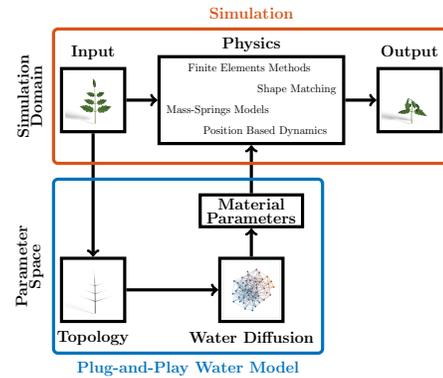
**Figure 2: The water diffusion model we propose is designed to be a plug-and-play extension to different kinds of physical simulators. By using the topology of the simulated plant, it can compute the complex behavior of the water diffusion inside the plant itself. The water distribution is then used by the physical simulation to compute wilting deformations more realistically than those obtained by the manual tuning of the plant’s stiffness.**
