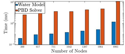
**Figure 11:** Distribution of the average execution time between the water model (blue) and the PBD solver (orange) at every time step for different plants. The PBD solver is computationally dominant independently on the number of nodes. The experiments have been carried out on a machine equipped with an Intel i7-10700K CPU and 32 GB of main memory.
