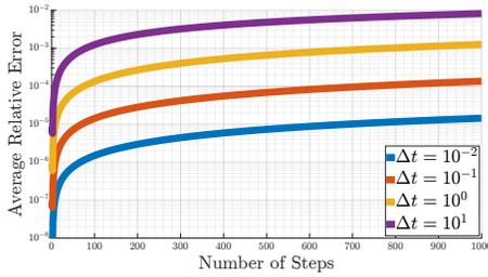
**Figure 4: Relative mean squared error of the solution obtained with BDF6 over time, compared with the analytic solution and averaged across plants with different resolutions. Each curve is obtained by selecting a different time step for the integration.**
